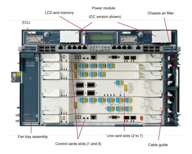
Figure 2. Cisco ONS 15454 M6 MSTP Modules
