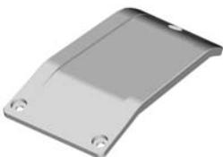
*Our 600 series skid shoes have a raised rib on both edges for extra long wear. In this raised area the shoe is 1/2" thick. The rest of the skid shoe is 3/8" thick. This is a very high density UHMW poly for extra wear.*
