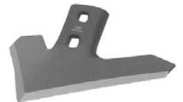
**ORDERING INFORMATION:** All WCC series sweeps are 47 degree with a 1-3/4" bolt hole spacing. Bolt hole size is 7/16". This configuration fits most field cultivators and soil conditioners including John Deere (built 1986 and later), IH, Case-IH, Sunflower, White, Wilrich, Kewanee, Kent, Landoll, M & W, New Holland, and others.
