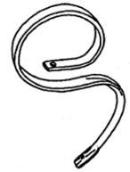
Ground clearance is measured from the mounting hole to the sweep bolt hole.
