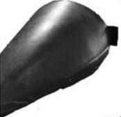
KCFSR90E  | <b>Poly wear strip</b> to repair damaged snouts. Fits JD 90 series with serial number prior to 695300. Kit includes 1 RH and 1 LH poly strip and mounting hardware. | 79315 | \$19.95    |
