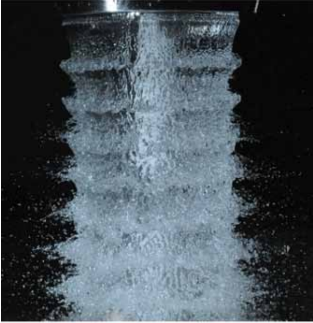
FIGURE 7 Image of a cavitating jet in air ( d = 1 mm, p_1 = 30 MPa)
