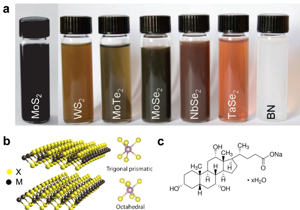
Fig. 40. Dispersion of nanosheets of transition metal chalcogenides and BN in aqueous solution requires the use of surfactants such as sodium cholate or SDS. (a) Photograph of dispersions of MoS 2 , WS 2 , MoTe 2 , MoSe 2 , NbSe 2 , TaSe 2 , and BN stabilized in water by sodium cholate. The powders were sonicated at initial concentration, C_i = 5 mg/ml, with a surfactant of concentration C(SC) = 1.5 mg/mL for 30 min. (b) Chemical structure of two layers of a transition metal dichalcogenide where M is the transition element and X the chalcogen. Two polytypes of single-layers are shown: trigonal prismatic (D 3h ) and octahedral (D 3d ). (c) Sodium cholate. (Reproduced with permission from Refs. [392,390].)
