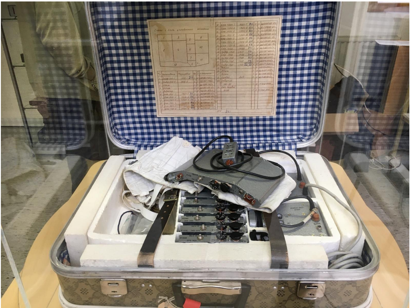
An East German bug girdle with receiver in a suitcase. Below: UK bugs.
