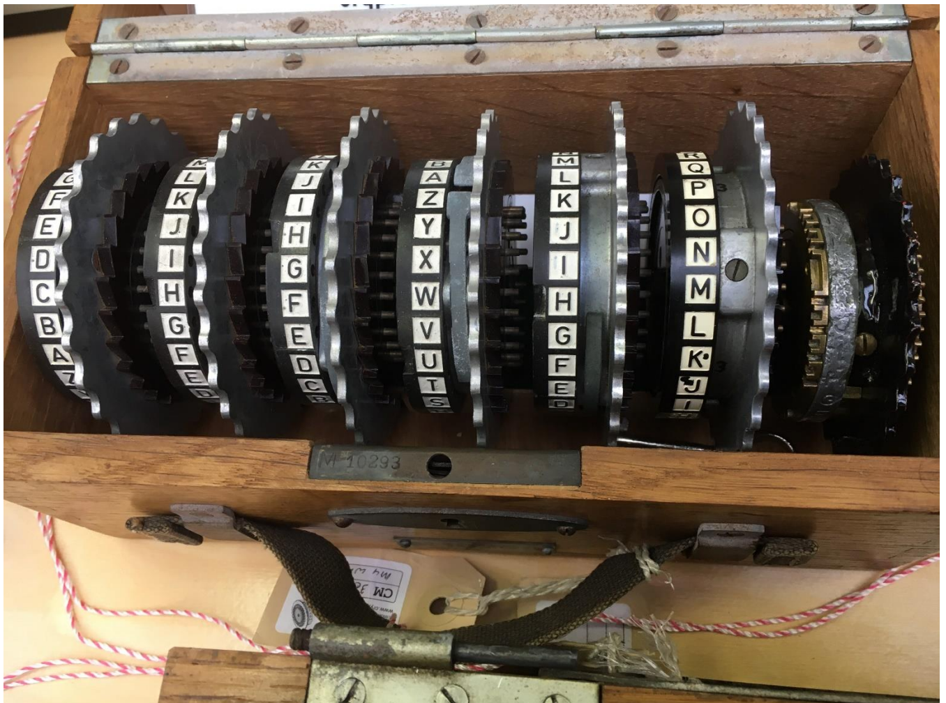
Above: ENIGMA K machine and the KG-84 dedicated loop encryption device for digital data. Below: ENIGMA wheels
