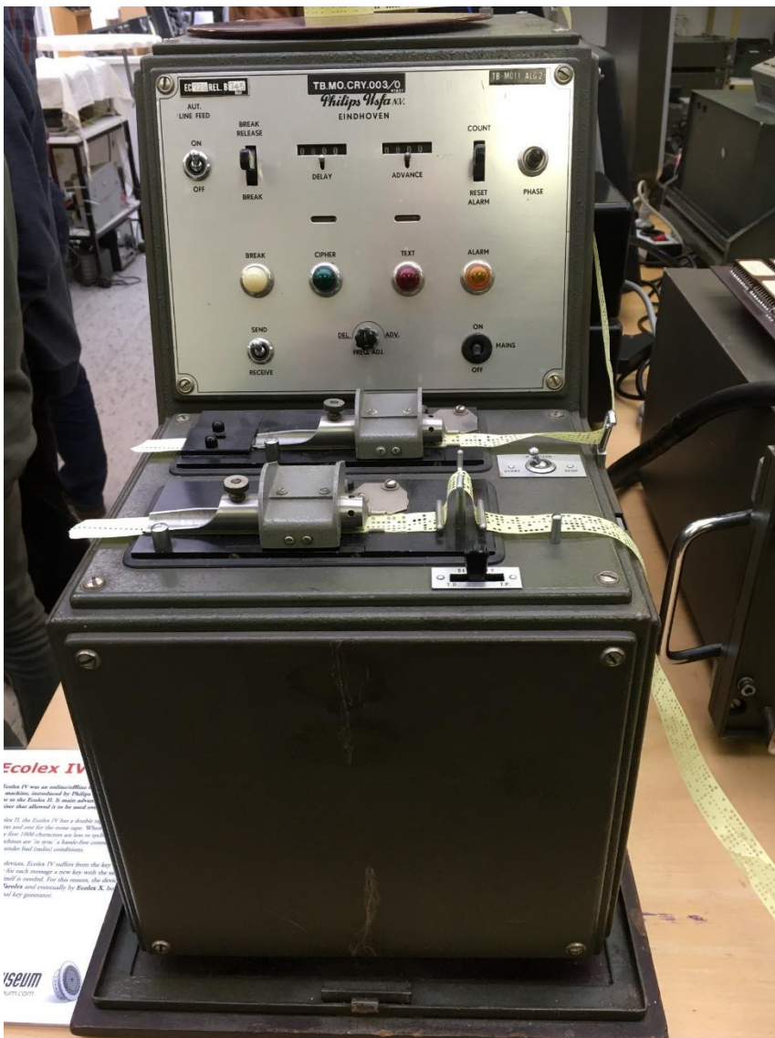
Ecolex online/offline One-Time Tape (OTT) cipher machine
