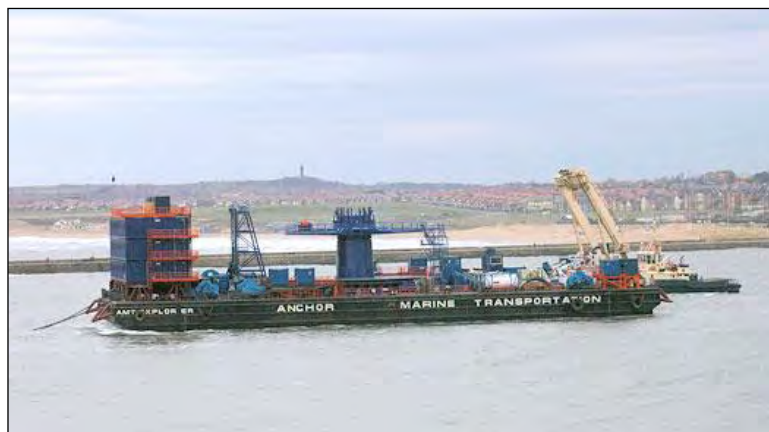
Plate 4. Typical cable lay barge
