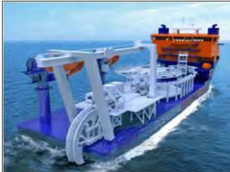
Plate 3. Typical cable installation vessel
