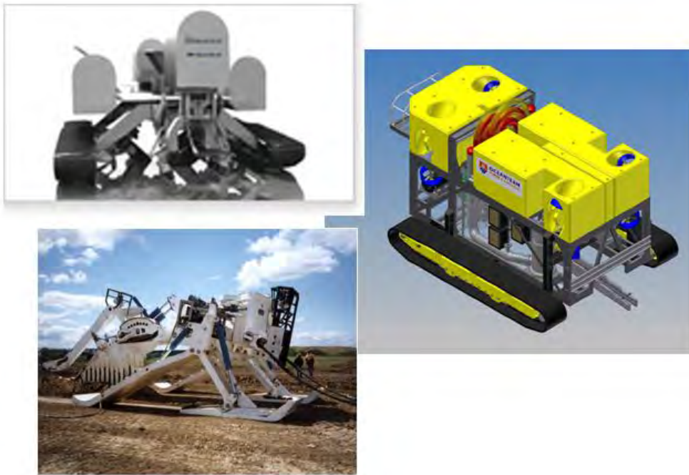
Plate 2. Jetting Trencher (right), Mechanical Trencher (upper left) and Cable Plough (lower left) equipment used in typical subsea cable burial operations
