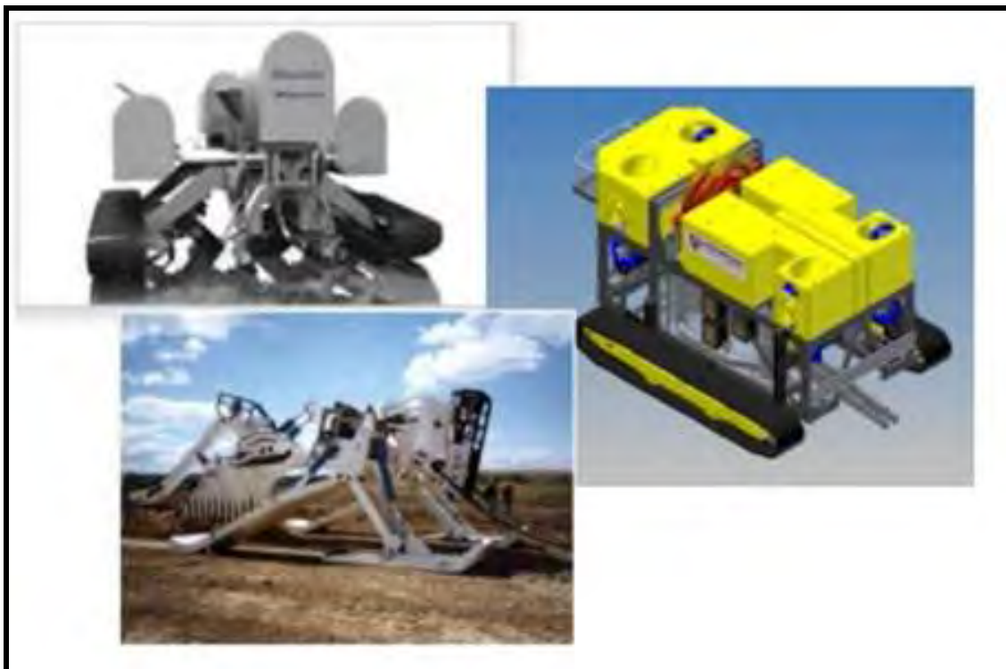
Jetting Trencher (right), Mechanical Trencher (upper left) and Cable Plough (bottom left)
