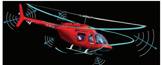
Fig.3 Helicopter noise sources [5]
