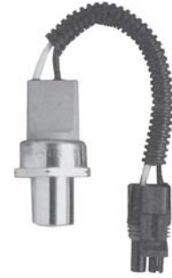
1390 Weatherpak High pressure, normally closed Open: 250 psi, Close: 210 psi 1/4" Female Flare, R12/R134a
