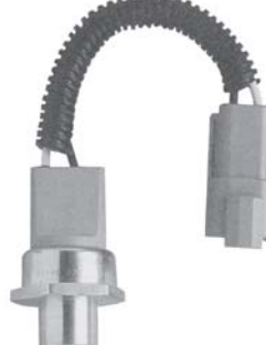
1389 Deutsch High pressure, normally closed Open: 275 psi, Close: 235 psi 1/4" Female Flare, R12/R134a
