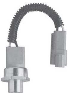
1387 Deutsch High pressure, normally closed Open: 300 psi, Close: 250 psi 1/4" Female Flare, R12/R134a
