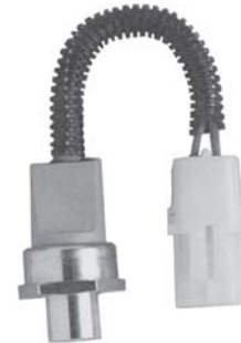
1380 Weatherpak High pressure, normally closed Open: 275 psi, Close: 235 psi 1/4" Female Flare, R12 Only
