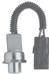
1371 Weatherpak Low pressure, normally open Open: 8 psi, Close: 34 psi 1/4" Female Flare, R12 Only
