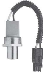
1385 Weatherpak High pressure, normally closed Open: 300 psi, Close 260 psi M10 Female Schrader, R134a
