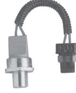
1386 Metri-Pak High pressure, normally closed Open: 325 psi, Close: 275 psi M10 Female Schrader, R134a
