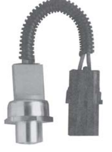
1388 Weatherpak High pressure, normally closed Open: 300/325psi, Close: 220 psi 1/4" Female Flare, R12/R134a
