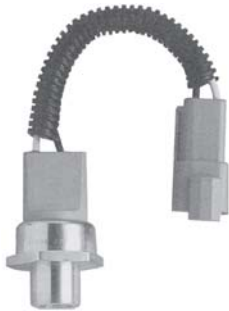
1383 Deutsch High pressure, normally closed Open: 250 psi, Close: 210 psi M10 Female Schrader, R12 Only
