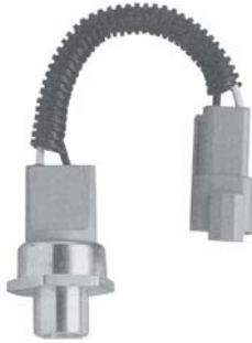
1384 Deutsch High pressure, normally closed Open: 300 psi, Close: 265 psi M10 Female Schrader, R134a
