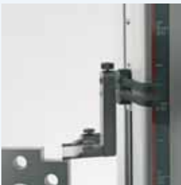
Probe contact with the motorized measuring carriage.
