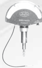
Millimess precision probe, constructed in 1937. First indicating unit for reliably recording dimensional differences down to 1/1,000 mm
