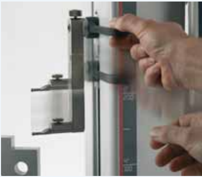
Ill. 1. Move the measuring carriage by hand in the direction of the object to be measured.
