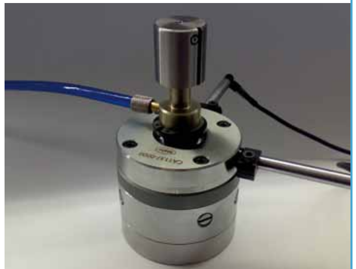
Jet air plug gage mounted on a floating bearing with position query to diameter and determination of position
