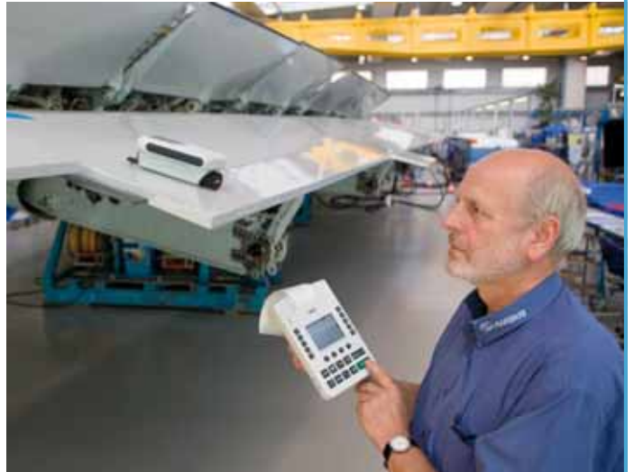
Roughness measurement on wings (Airbus)
