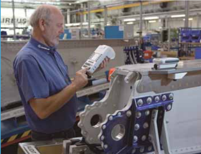
Roughness measurements on flap tracks (for landing flaps) (Airbus)
