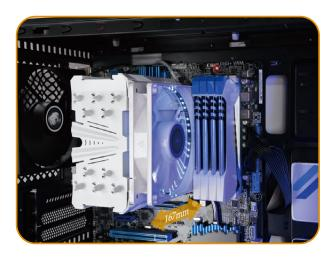
Supports CPU cooler up to 167mm in height
