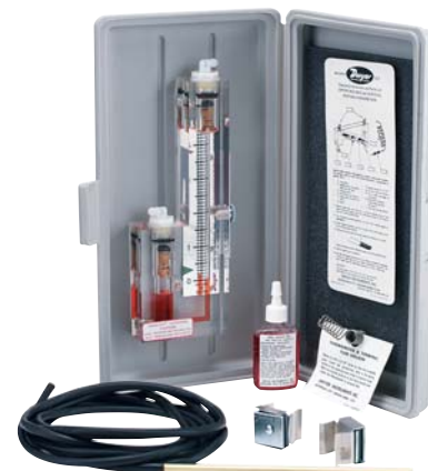
Fig. 4-3. No. 104 solid plastic portable vertical manometer shown attached to inside of carrying case cover. Gage may also be removed from case and used in standing position or attached to any vertical steel surface with magnetic clips provided.
