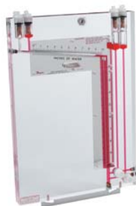
Fig. 8-2. Typical of Series 420 Inclined-Vertical Manometers is this No. 422-10 double column manometer with a total range of 0 to 10" of water. Single column models are also furnished. Design features are essentially the same as for the Series 424. They are accurate to \pm 1\% and are particularly suited for use with pitot tubes and in flow measurement or similar applications.
