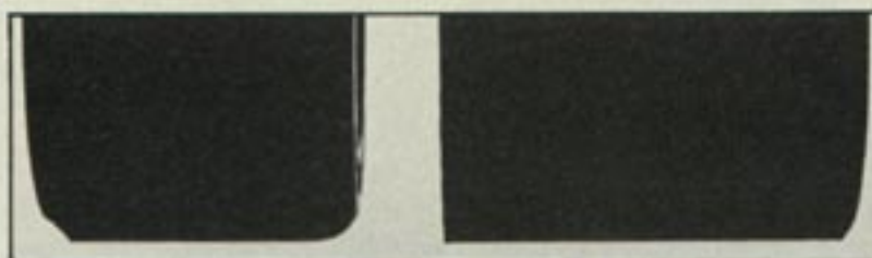
Contrasting contact widths (both wheels are 65mm diameter) Left: 55mm, Right: 36mm
