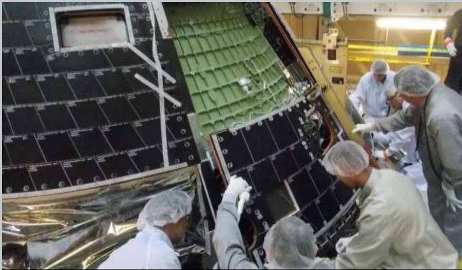
Back Shell Installation
