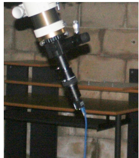
Figure 2. Left: Speckle Interferometry installation on the Kuhn 22" Telescope. A single blue USB3.0 cable connects the camera to the laptop on the white table at lower right. Right: Close-up of the simple finding and magnification optics: an illuminated reticle eyepiece is at top in the flip mirror; below are the Baader Hyperion 10mm eyepiece, projection tubes, and tiny (30mm cube) camera, attached to the blue USB3.0 cable. No filter wheel was used in this early configuration.
