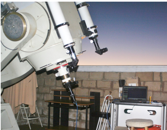
Figure 2. Left: Speckle Interferometry installation on the Kuhn 22" Telescope. A single blue USB3.0 cable connects the camera to the laptop on the white table at lower right. Right: Close-up of the simple finding and magnification optics: an illuminated reticle eyepiece is at top in the flip mirror; below are the Baader Hyperion 10mm eyepiece, projection tubes, and tiny (30mm cube) camera, attached to the blue USB3.0 cable. No filter wheel was used in this early configuration.
