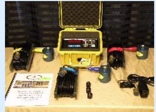
Digital Indication, three load cell transducers and one inch mounting
