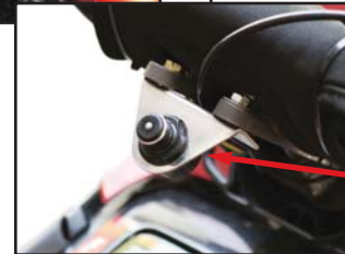
Aftermarket Bars Installed - OEM Protective Cover No Longer Fits
