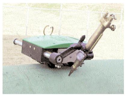
Pipe diameter 16" / 406mm and larger can be cut parallel to the pipe axis.
