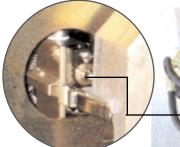
Blade Shut-Off Device does not allow the machine to be operated until the Blade Guard is locked into position.
