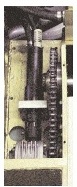
The Blade Speed and Forward Motion are held constant by the Powerful *Heavy-Duty Pneumatic Motor Drive and a Heavy-Duty Transmission*.
