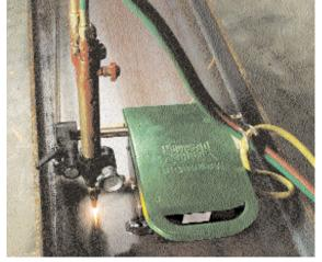
Vertical or Horizontal I Beam 20" wide or wider can be precision cut with MagnaCut.
