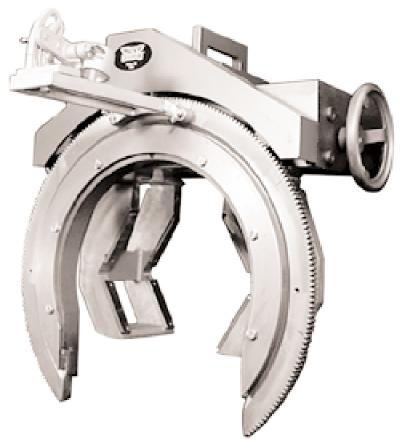
Made from *aircraft quality aluminum*, the Super II was designed to handle most fabrication shop applications. The unique self-centering jaws of the Super II accurately center the machine on any tubing or pipe having a diameter of 2 3/8" - 12 3/4" / 60 - 324mm.
