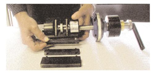
Porta-Mill is easily and quickly changed from one pipe to another by changing the Mandrel Leg.
