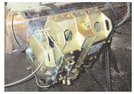
The Heavy-Duty Air Motor of the Pneumatic CGM-1 allows the machine to cut pipes regardless of diameter in a minimum amount of time and effort.
