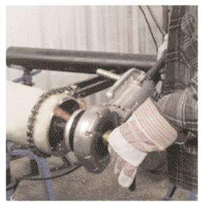
Ideal for fast set-up and facing and beveling of stainless steel and other nonferrous pipes.
