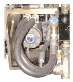
Hydraulic force applied to the Hydraulic Motor insures constant speed of the Cutting and Beveling Blades and rotation of the machine around the pipe.
