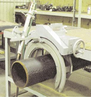
The Super II can be attached to a fixture or table and the pipe move through the jaws. The Super II is an excellent cutting machine for pipe yards—when used in conjunction with a Jib Crane or Forklift
