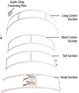
Guide Strip Add or remove Guide Strip sections as needed when changing pipe diameters.
