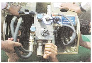
The Controls of the Pneumatic and Hydraulic CGM-1, that Control Blade Speed and Machine Speed and Direction, are within easy reach of the operator.
