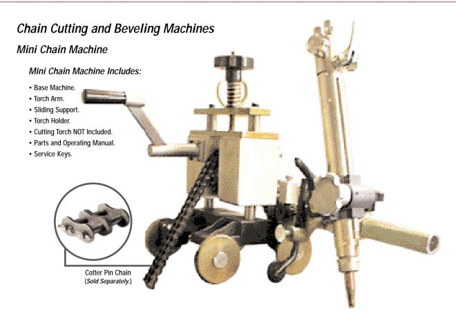
Most popular of the Chain Machines, the Lightweight Mini Chain Machine is recommended for cutting random lots of small or larger diameters of pipe. Easily adjustable from one pipe size to another, the Mini follows the pipe outside diameter to produce a consistent bevel. The *compact unit* reduces down time and maintenance cost. The Mini Chain Machine's unique design delivers exceptional performance and maximum results. Cuts pipe diameters from 2" / 51mm to unlimited. *CE Approved.*
