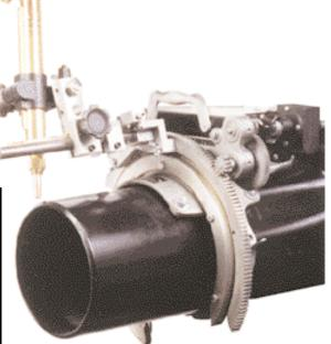
The PRO Model with Base Unit, used in conjunction with the Motorized Saddle Machine, reduces grinding time by 85%.
