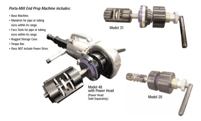
Ror counterbore pipe ends. The Steel Mandrel Assembly of the Porta-Mill expands against the inside diameter of the pipe providing a solid mounting for smoother extremely accurate bevels. Inexperienced welders and pipefitters with little or no training can achieve precise bevels and lands in minutes. Porta-Mill's superior design makes it an exceptional performer having the utmost durability. Models are available for inside diameter from 1.6" / 41mm to 8.125" / 206mm.
