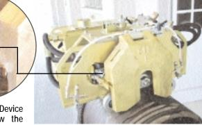
Adjustable Jets of the Heavy-Duty Mist Lubrication System Direct Coolant at Cutting and Beveling Blades to achieve *maximum blade life*.
