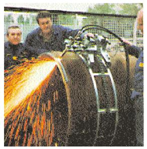
Guide Strip Part No. 05-520-013 Guide Strip insures a precise square cut on 18" / 457mm and larger pipes.
