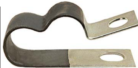
.69 x .69 TUBES .75 W x 2.56 L .40 HOLE OGS, 383701-S S8/RUBBER
