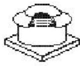
Screen on Roof Ventilator
