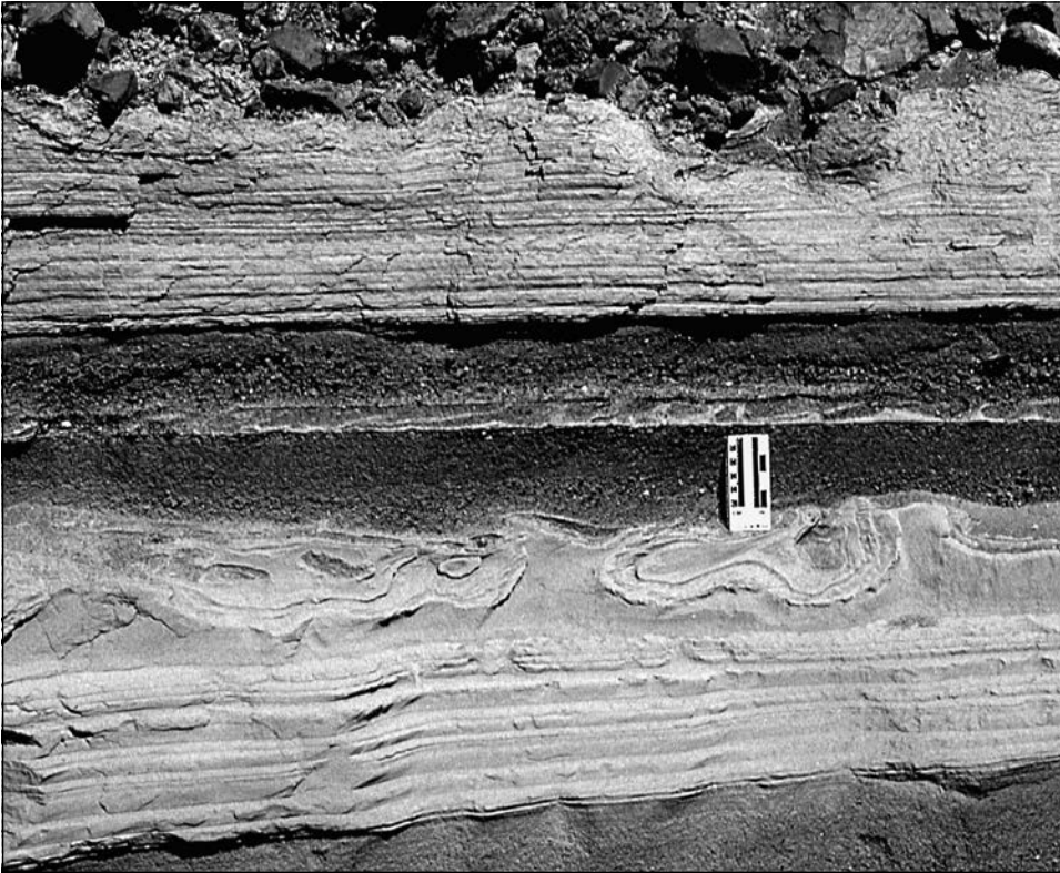
Figure 51. Contrasting texture and deformation in light-colored FD layers in section 3 (top of flood bed 9 and flood bed 13 within flood sequence III) (Fig. 47). The lower FD interval has coarser grain size and thicker beds (“member b” in Fig. 50) than the upper interval (“member d”). Soft-sediment deformation by loading of coarser sediment is much more intense in the lower bed, within the flood sequence, than in the upper bed, interpreted to mark the top of the flood sequence with a hiatus prior to deposition of overlying gravel. Scale bar is 10 cm tall.
