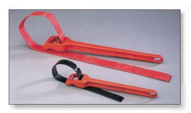
Strap Wrench handles are malleable iron and meet U.S. Govt. mil spec GGG-W-651-E type 5. Strap Wrenches are available in two handle lengths and three strap lengths. All straps are replaceable and are polyurethane coated to provide a non slip grip while preventing marring of chrome, brass, plastic and other hard to grip items.
