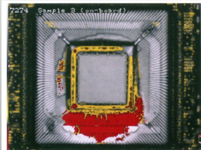
Figure 1 C-SAM image of a PEM, showing severe package cracking and delamination (red). This part was imaged while still on the board.
