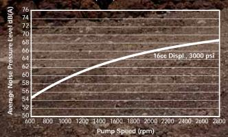
It's a fact of life. Mechanical equipment makes noise. Some noise is unavoidable, such as when hardened materials make sudden contact. Other kinds of unwanted sound, such as airborne noise from hydraulic vibration, can be reduced through design improvements. Eaton gear pumps provide high performance at lower decibel levels, which reduces operator fatigue and provides better working conditions for employees and visitors.
