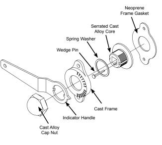
•All SR and SRH type regulators include a cast alloy frame and a neoprene frame gasket.
