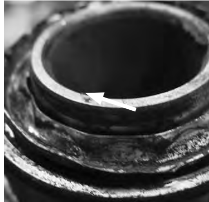
Distorted seal due to interference with adjacent mating parts.
