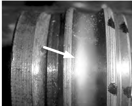
Fine particle abrasive wear on the inner race, commonly known as 'frosting'.
