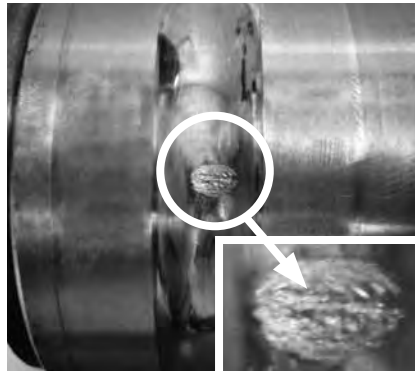
Inclusion origin: spalling from oxides or other hard inclusions in bearing steel.
