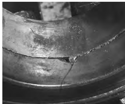
Inner ring cracking due to excessive taper on the shaft.
