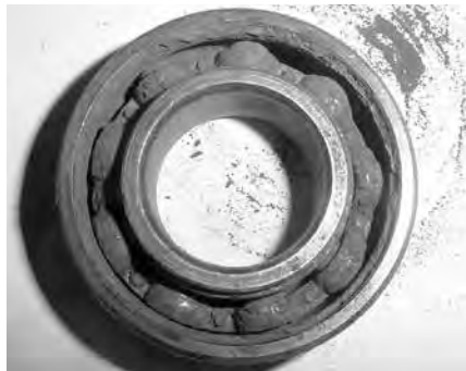
Gross contamination resulting from harsh operating conditions and/or seal failure.
