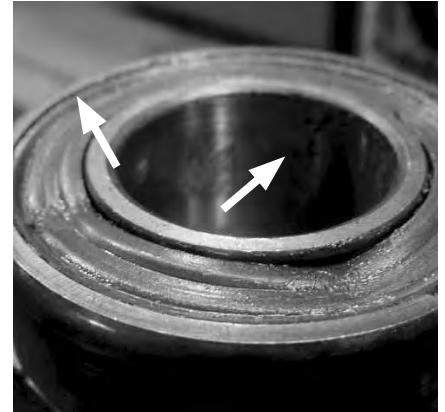
Seal damage due to improper installation procedure and/or tools.
