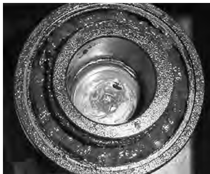
Lubrication characteristics of the grease are compromised by water ingress.
