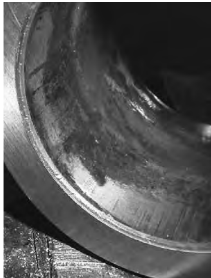
Fretting on inner ring due to out-of-round shaft.
