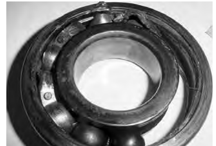
Metal cage damage due to misalignment or excessive speed.
