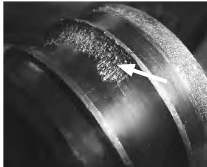
Geometric stress concentration (GSC): spalling from misalignment, system deflections or heavy loading.
