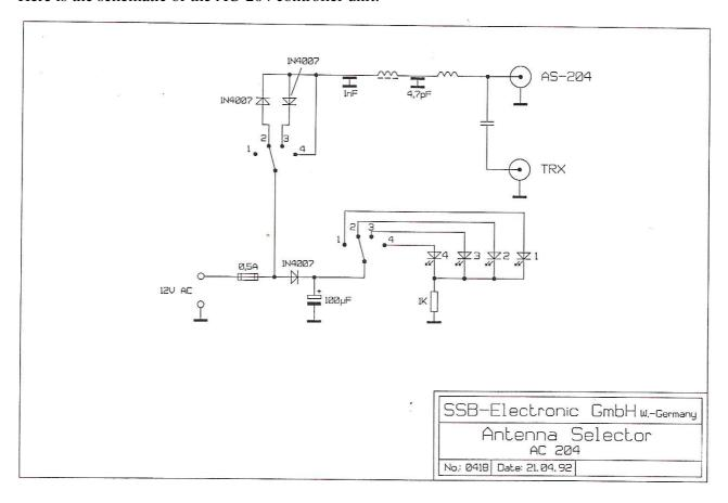
Here is the schematic of the AS-204 remote antenna switch unit:
