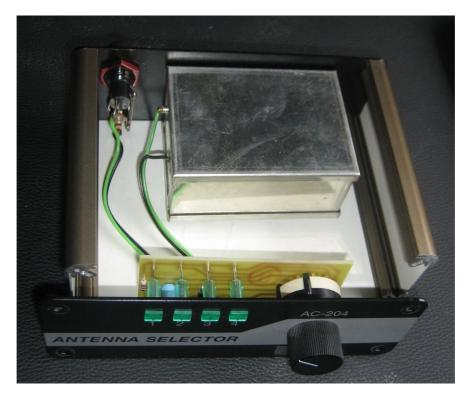
Finally here are detailed pictures of the AS-204 remote antenna switch including how it looks inside:
