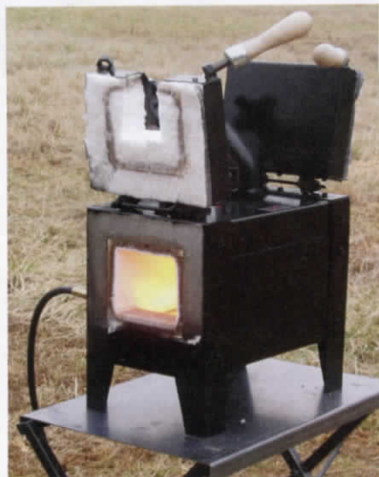
NC Tool Co.'s Knifemaker Gas Forge is specifically designed for forging damascus and single-steel knife blades, showcasing insulated doors on both ends, an exhaust port, a 13.5-inch firebox, high-efficiency burners, push-button ignition and uniform heating of up to 2,350°F.
