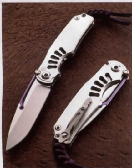
The lock bar of the Chris Reeve Knives Ti-Lock is mounted along the back of the blade toward the pivot. When the blade is opened, the handle edge of the lock bar, which has a cross bar with thumb-stud-like grips, is forced down into a slot through spring pressure, locking the knife securely open. (Point Seven photo)
