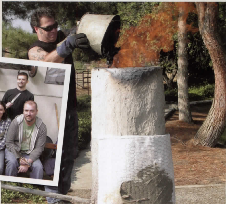
David Mirabile fuels the forge fire for making Japanese tamahagane steel at the California Hammer-in in Visalia, California. (photo courtesy of Michael and Marcie Vagnino)
