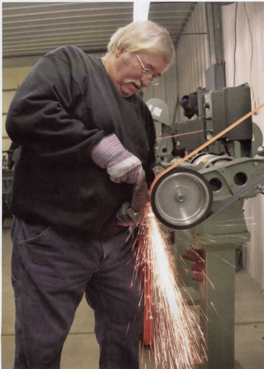
Tom McGinnis of Ozark Knife Makers, a Burr King dealer, uses the Burr King 960-272 grinder with a 1.5-horsepower Baldor motor and a variable-speed controller. (James Krier photo)
