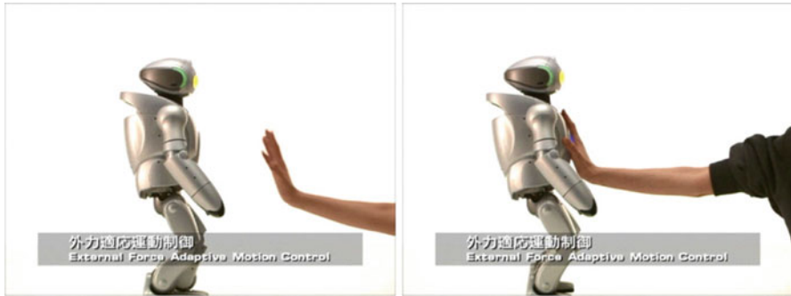
Fig. 8 External force adaptation motion control
