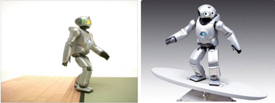
Fig. 7 Walking on uneven or moving terrain using terrain adaptive motion control
