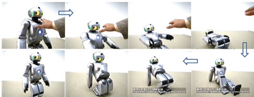
Fig. 9 Integrated adaptive fall-over motion control
