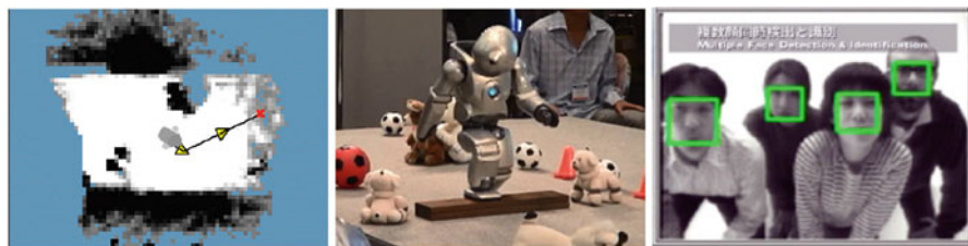
Fig. 14 Examples of intelligent functions – path planning on occupancy grid ( left ), obstacle avoidance using it ( middle ), and face detection ( right )
