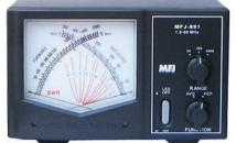
MFJ-891 SWR less than 1.2:1. **\$10995** Meter accuracy is +/- 10% of Ship Code A full scale or better. Has lighted meter on/off switch.
