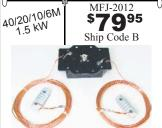
MFJ-2012 Power-Lite<sup>™</sup> 40/ 20/10/6 Meters, handles 1500 Watts PEP CW/SSB. 67' long overall, long leg 44.6, short leg is 22.5 feet. Robust high-power version of the MFJ-2010 with 14-guage stranded-copper wire and porcelain end insulators. Pull-tested to 200 pounds.
