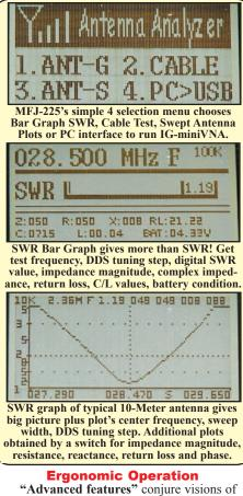
greater complexity and more buttons to push . . . not true for MFJ-225! The graphic display is *"advanced"* because it places more information at your fingertips without needless scrolling and searching. Also, the layout is unique with three large soft-touch selector buttons located on the front panel next to the screen and a large side-mounted
