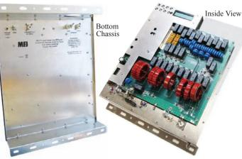
Automatic inductor and capacitor limiting prevents tuning extreme loads which can destroy your tuner.
