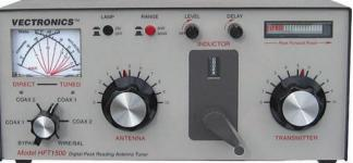
ceramic. Coax 1 is for tuned and funer bypass; Coax 2 is for tuned and tuner bypass, bypass and balanced antenna.
