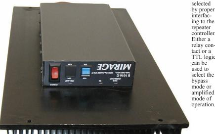
interfacing to the repeater controller. Either a relay contact or a TTL logic can be used to select the bypass mode or amplified mode of operation.
