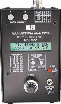
Together, these functions are extremely useful for checking the operation of oscillators, transmitters, as well as assessing the strength of radiated signals from antenna arrays.
