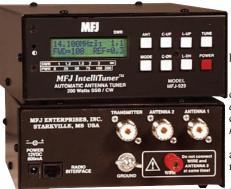
The MFJ-929 IntelliTuner-Compact<sup>™</sup> lets you automatically tune any coax fed or random wire antenna 1.8-30 MHz at full 200 Watts SSB/CW. It can match 6-1600 Ohms (SWR up to 32:1) - - that's a 50% wider matching range at a higher power level than lesser competing products.
