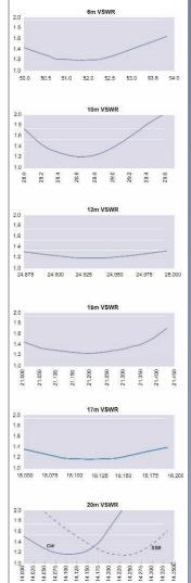
The R-6000 employs quarter wavelength stubs on 10 and 15 Meters to replace standard trap coils. The result is lower loss and wider bandwidth. The R-6000 covers all bands 6 through 15 meters at a VSWR under 2:1. On 20 meters you can select the top 300 KHz or bottom 300 KHz of the band.
