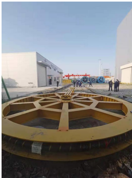
Figure 10 Tensile bending test of the 3x 1200 mm 2 38/66 (72.5) kV XLPE submarine power cable around a 6.0 m sheave
