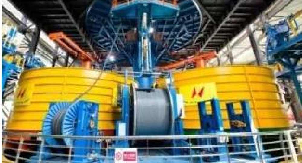
Figure 5 SKET Laying-up system
