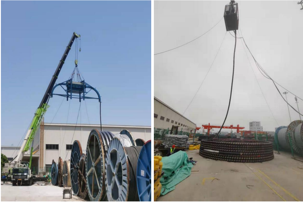
Figure 9 Coiling test of the 3x 1200 mm 2 38/66 (72.5) kV XLPE submarine power cable into a fixed static tank
