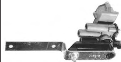
HEIGHT CONTROL VALVE
