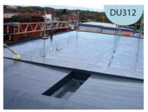
totally seamless waterproof surface on prepared concrete and can be applied by squeegee, brush, trowel or roller. The two-component polyurea formulation is suitable for waterproofing pitched or flat roofs, decks and balconies and other areas where a degree of flexibility is required. The trafficable, cured surface also makes it suitable for waterproofing concrete floors in car parks, for example.
