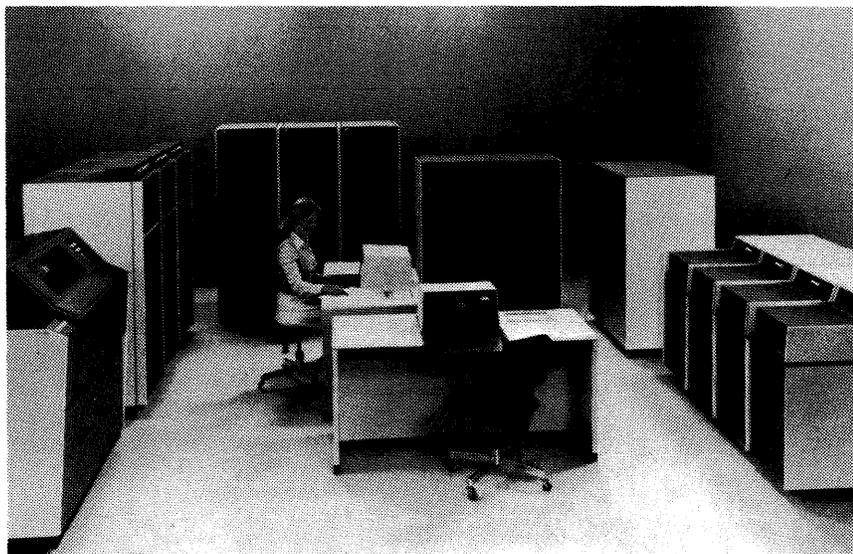
*NCR's V-8500 Group II Series includes five models that can have from one to four CPUs, 1 to 16 megabytes of memory, and a wide range of I/O devices. Performance is comparable to the IBM 4300 Series.*
