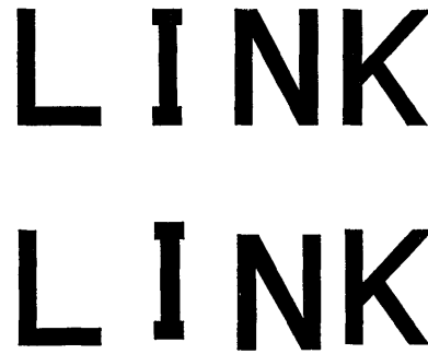
Fig. 7—Normal printing and 0.005-inch misalignment above and below a line.
