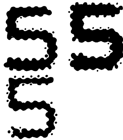
Fig. 2—Character line widths and noise vary greatly with inking and impression.
