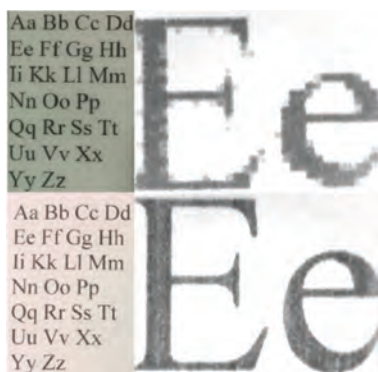
Fig. 8. Top image: 2.71" vertically oriented display; bottom image: regular paper. A normal view is shown on the left and a 50x magnification using a USB Delta Optical DO Smart microscope on the right.
