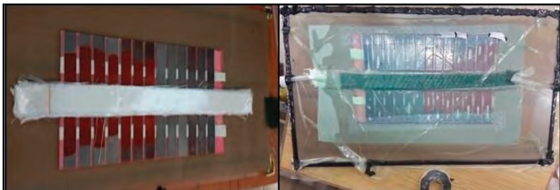
Fig. 3. Specimen fabrication with vacuum bagging technique
