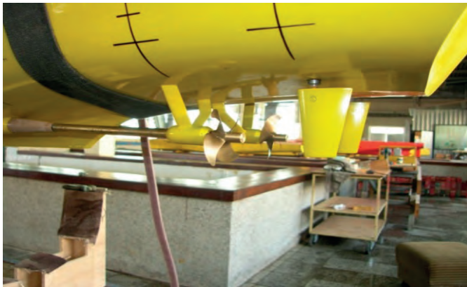
Fig. 5. View showing the arrangement of rudders and propellers
