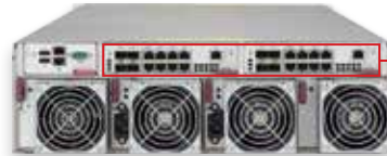
MBE-314E-416/420 or MBE-314E-816/820 (3U MicroBlade Rear View)
