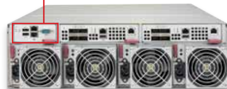
MBE-314E 3U MicroBlade Enclosure Rear View
