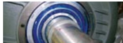
Oversized NSK/SKF bearings with Polyrex EM grease
