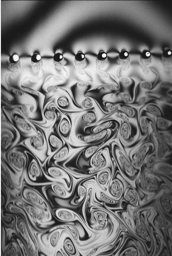
Figure 2. Two-dimensional turbulent flow visualized in a soap film by Maarten Rutgers—for an even more striking illustration of this phenomenon, see the video clip under the “Turbulence” section of http://maartenrutgers.org/ [20].
