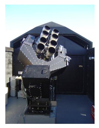
Figure 3.1: Photo showing the SuperWASP instrument, its robototic mount supports eight 11.1 cm refractive telescopes. We also see the roof which automatically opens and closes. Photo courtesy www.superwasp.org.
