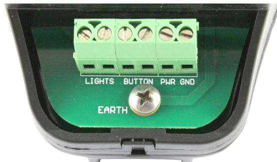
6-Wire System Termination View
