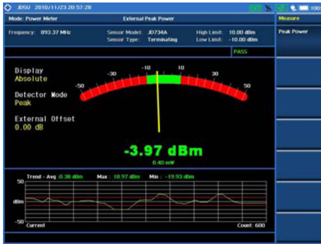
External Power Measurement
