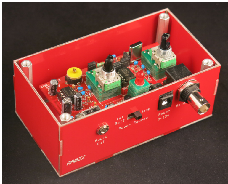
Figure 6.1 – Board Mounted in Enclosure
