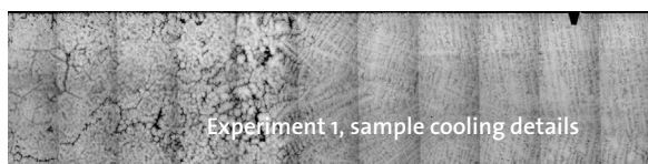
X-ray imaging (above and below) of TiAlNb sample processed on MAXUS8, courtesy: ACCESS e.V. (Experiment 1)
