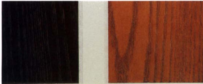
Ferrous sulfate over logwood dye
