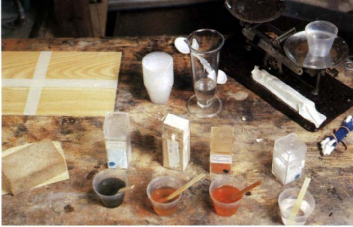
Your wood-dyeing experimentation kit needn't make your workbench look like Dr. Frankenstein's laboratory. The most important tools include: disposable mixing cups, mixing sticks and applicators; masks, goggles, gloves and other protective devices; and an accurate scale.
