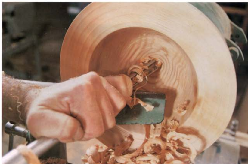
Top: The author shapes the outside of bowls from foot to rim with \frac{1}{2} -in. and \frac{3}{8} -in. deep-fluted bowl gouges. The tool's flute faces away from him as the left side of the tool shaves the green wood. Above: The right side of the cutting tool cuts the inside of the bowl.
