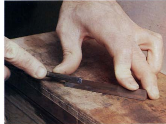
Above: Remove the burr that's raised in honing by inverting the parting tool over a slip stone and sliding it gently back and forth. Below: parting tools after sharpening, showing the rounded juncture where the two bevels meet (left), the inside corner, which is left sharp (center) and the bevel after polishing (right).
