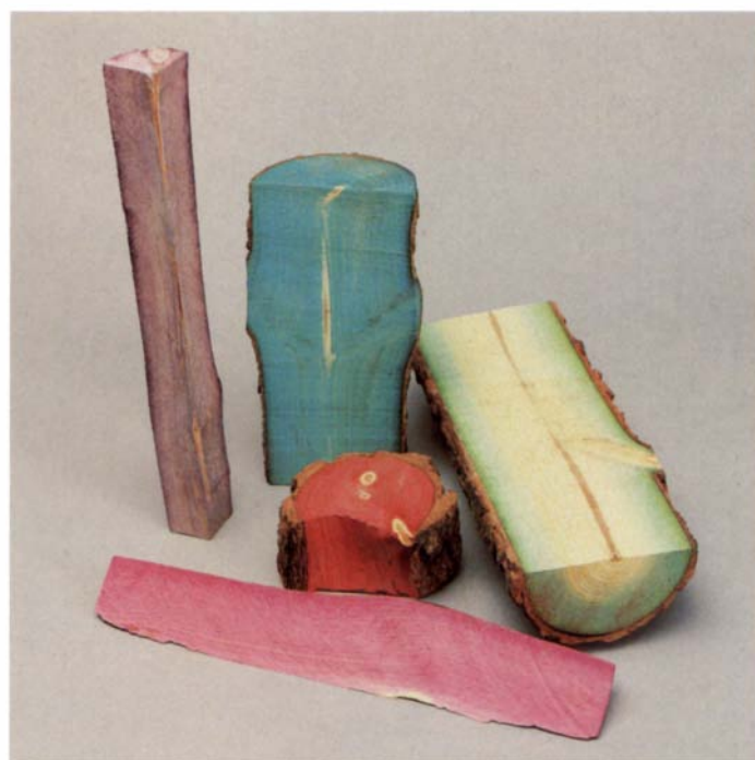
By letting a tree's natural circulation system absorb his pigmented solutions, LeRoy Frink is able to create a rainbow of unnaturally colored woods.
