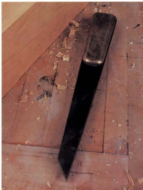
Author Podmaniczky designed his own mortising chisels and had them made. The chisels are fashioned from oil-hardened tool steel with bronze handles.
