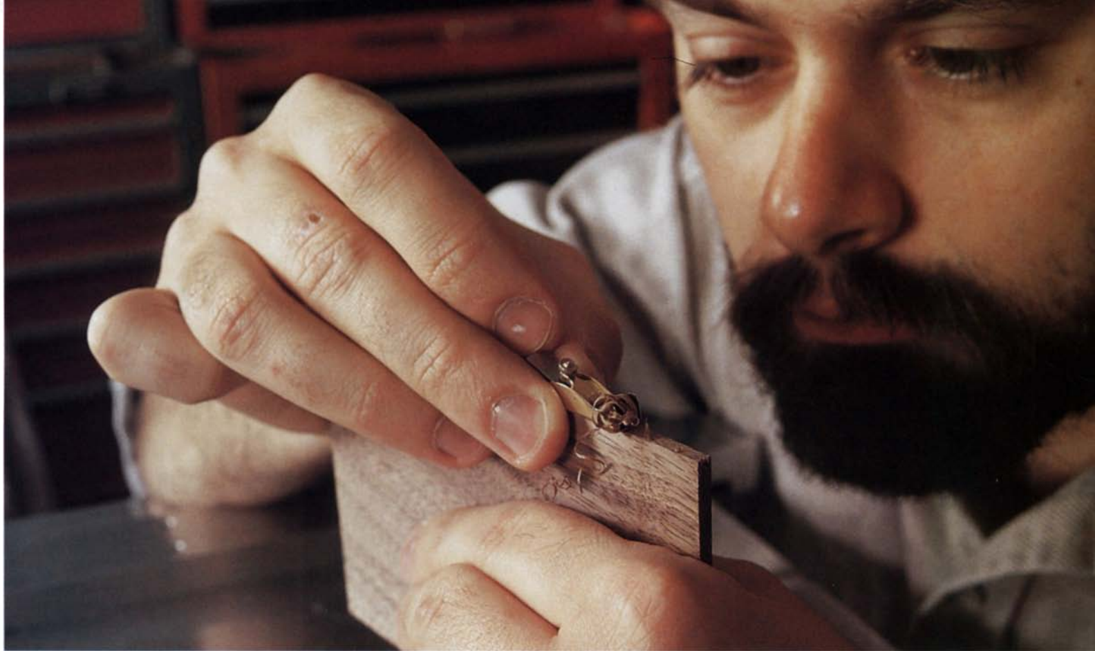
This tiny plane leaves scale-size tool marks on Robertson's miniatures, and is the handiest tool in his shop for truing edges.
