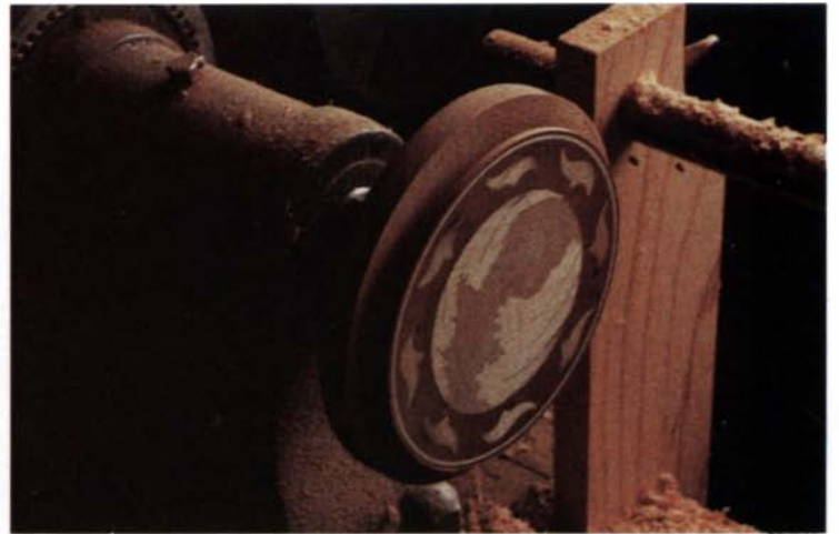
The cherry block is grooved and excavated, left, for the inlay. With the block attached to a faceplate, above, a shoulder is cut on the face to the final diameter of the pattern before a thin disc is cut off. The text below describes a safe tablesaw method, in which the block is left square, not turned round.
