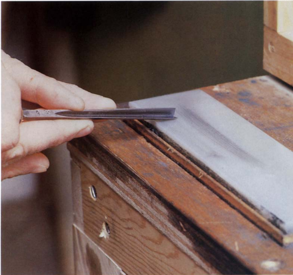
To hone a parting tool's bevel, lay one face flat on the benchstone and push or pull the tool along the stone. Lift the tool at the end of each stroke, and repeat the process. Note that the tool is held perpendicular to the length of the stone.
