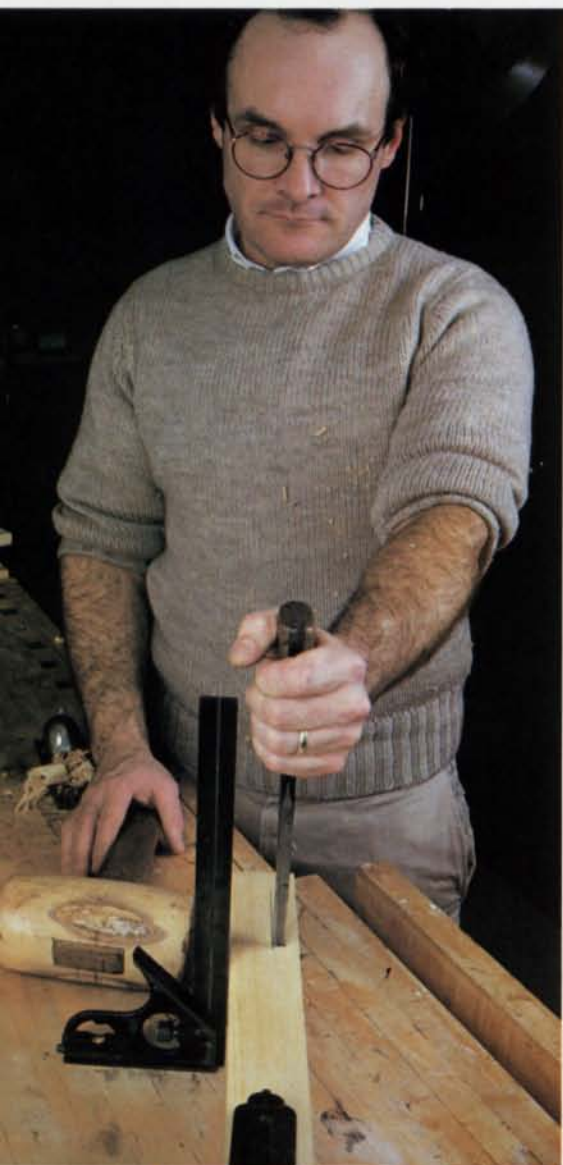
Top, marking out a mortise begins with setting the mortise-marking gauge to the width of the mortising chisel. Above, a square stood on the bench aids in keeping the chisel perpendicular to the work during chopping.
