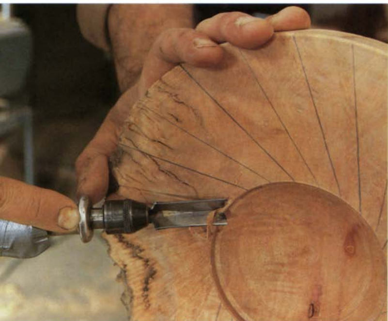
To lay out the rim design, Stirt bandsaws a piece of scrap to fit the rim, rotates a straightedge from it until he likes the angle (top), then glues the pieces together. The fixture is then moved around the bowl to mark the lines. Above, the thin lines along the rim of a cherry bowl are cut with a ½-in., 60° V-groove parting tool.
