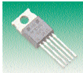
(b) SOT-263 Lead spacing 1.7
