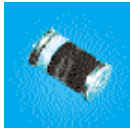
SOD80C (Mini-melf) L = 3.7, Dia. = 1.6 Grey band denotes cathode
