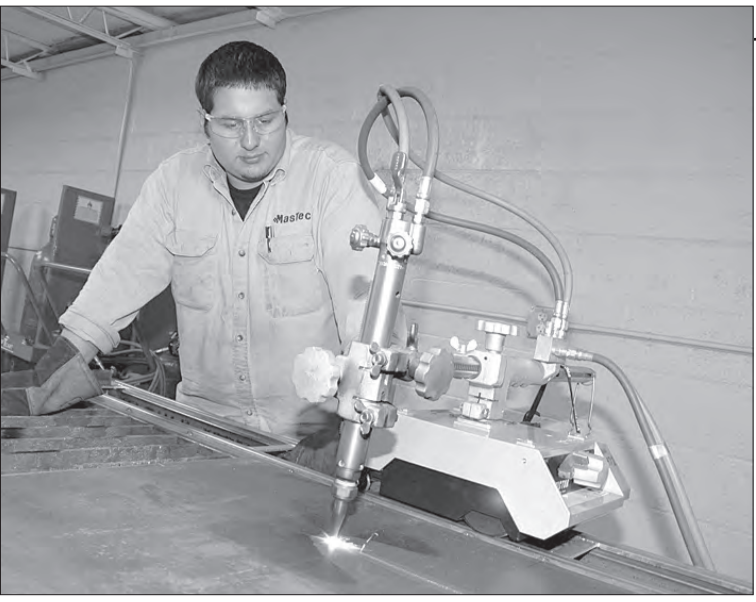
Chipola welding student, Nate Prietz cuts steel with a track torch.
