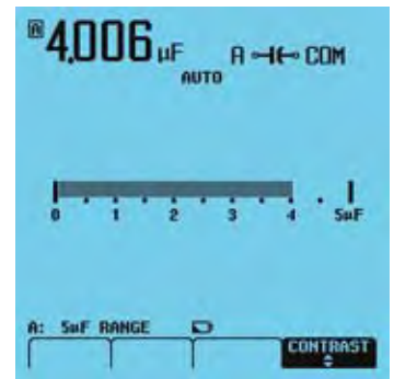
You can use the ScopeMeter 123 to check capacitance of a starting capacitor for a single phase motor
