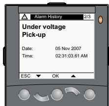
Alarm pick-up and drop-out.
