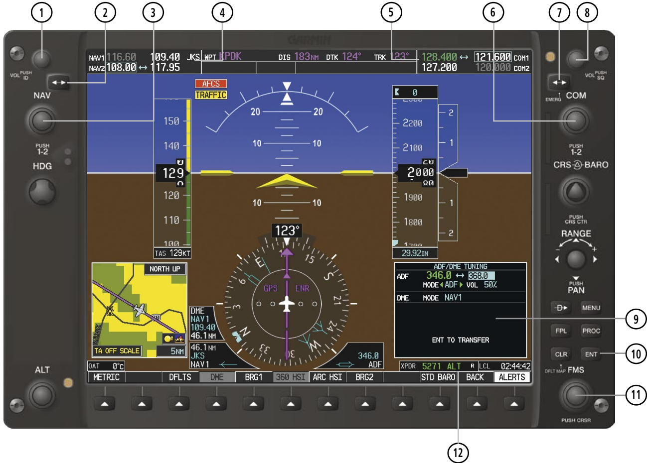
Figure 4-1 PFD/MFD Controls, COM/NAV Frequency Tuning Boxes, and ADF/DME Tuning Window (PFD Shown)
