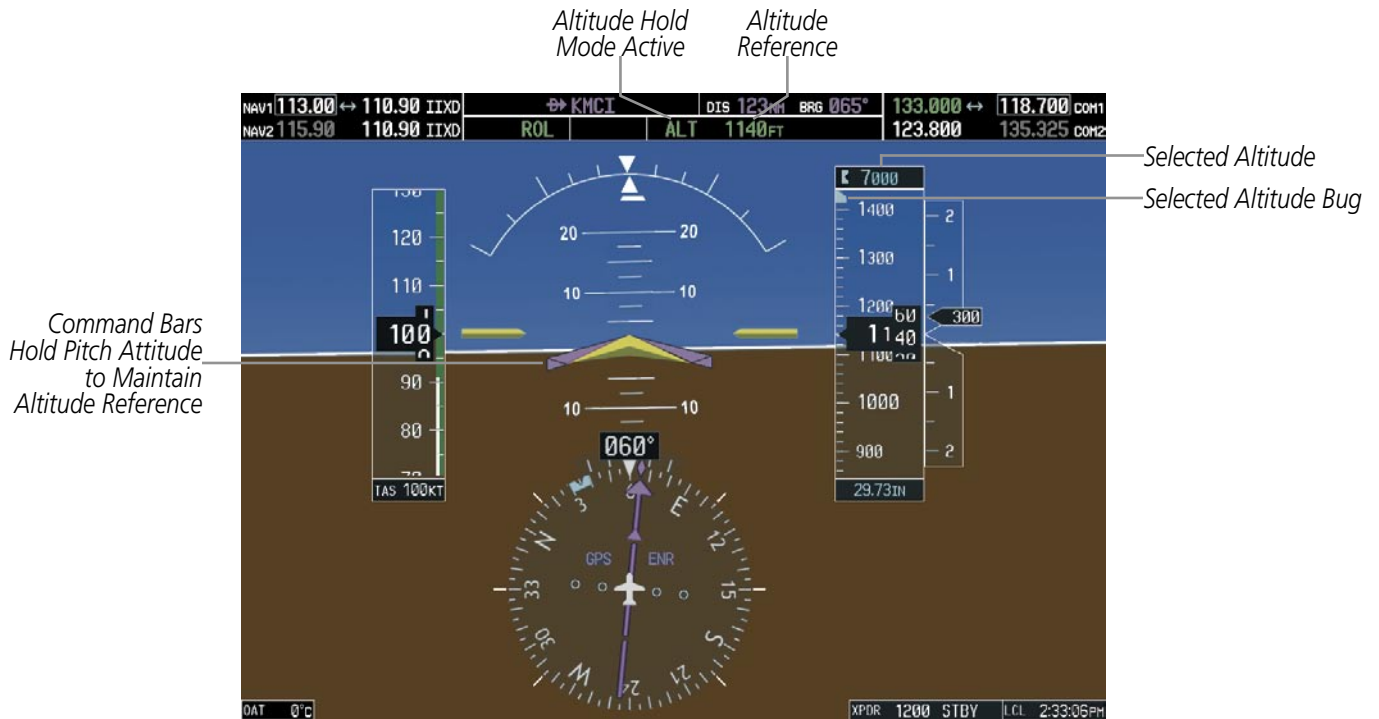
Figure 7-7 Altitude Hold Mode
