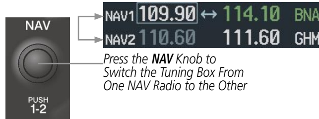
Figure 4-20 Switching NAV Tuning Boxes
